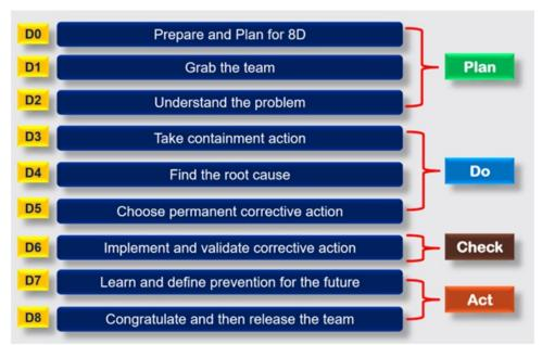
Fig. 3.4.2: How to Perform Root Cause Analysis
