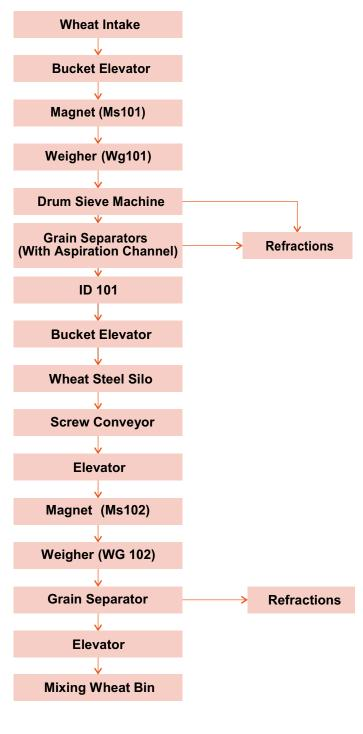
Fig. 2.2.4: Process Flow Chart of Wheat Cleaning System for Mill
