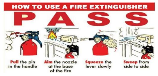
Fig. 5.7.2: Pass technique for Fire Extinguisher use
